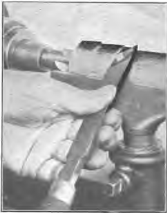
Fig. 21. Smoothing Up to a Shoulder.
